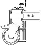
1iv Adjust outrigger variable height adjuster to ensure maximum contact with ground.
