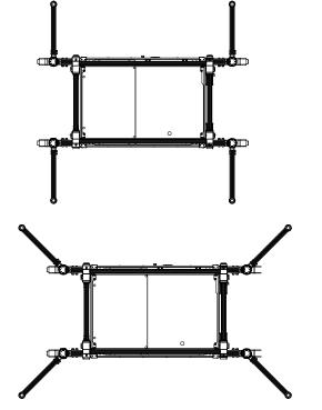
If the Razor Deck is to be used in a narrow high-sided aisle no outriggers are required.
