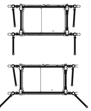
Each application will require an individual Risk Assessment. Ensure the work to be undertaken is considered. Where force is likely to be applied, deploy outriggers accordingly. Ensure the red adjustable section of the outrigger is firmly in contact with the ground.
