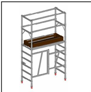
10. The toeboard set can now be placed on the platform, unfolded and positioned.
