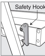
Wheel the Z600 Platform Steps to the work location and bring upright. Open out the steps until the platform is fully lowered and the safety hook has engaged. Next, deploy one of the stabilisers. Loosen the lock knob then lower the stabiliser until its foot is in contact with the ground then tighten the lock knob securely. Repeat this operation with the remaining stabiliser.
