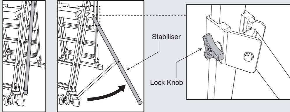
**DO NOT** set the stabilisers so that they raise the steps off the ground. The stabilisers are **NOT** designed to carry any weight.
