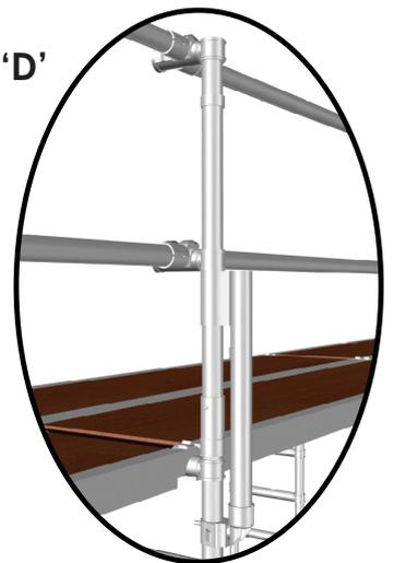
Detail D Installation of horizontals fitted to guardrail posts at top platform - Towers used in Facade
