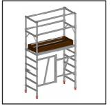
The toeboard set can now be placed on the platform, unfolded and positioned.
